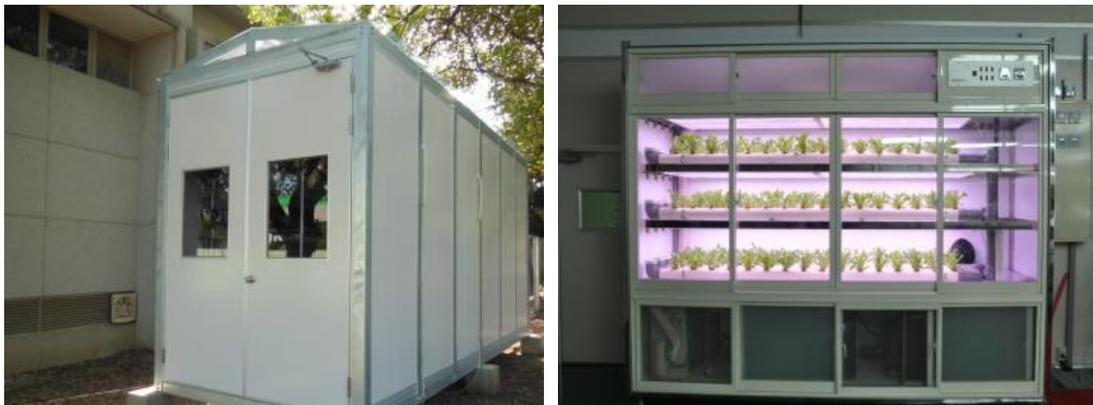
Two mobile types of plant factory, a two-compartment model growing lettuce and mushroom simultaneously in the same container (left) and a simply equipped model growing one single crop as a store showcase (right)
