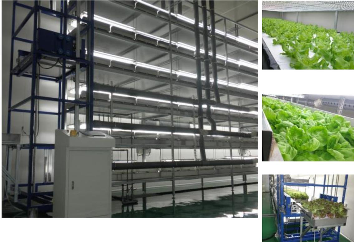
High-performance three-dimensional modular shelving system using artificial light source for a re-circulating water culture method
